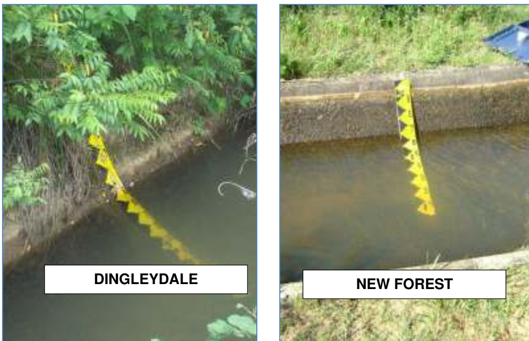
Figure 9.8 Installation of canal flow gauges
