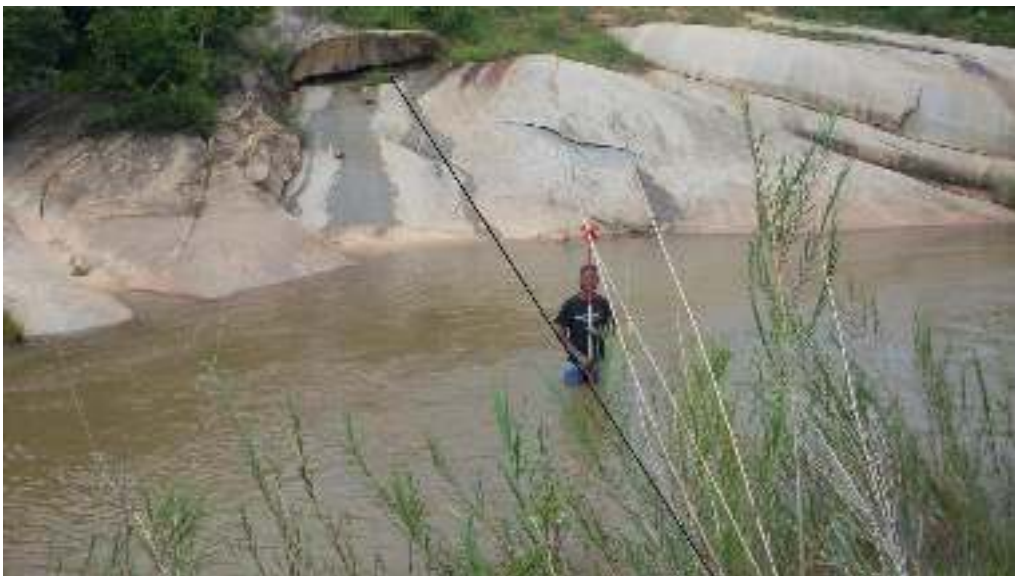
Figure 9.5 New Forest cross-section (black line) selected for rating streamflow gauge
