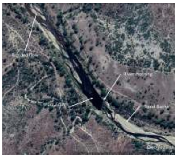
Figure 56: River crossing damming up flow
